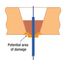
The diagram shows a specimen fully engaged in grip faces and grip faces not fully supported inside grip pockets. Arrangement can cause permanent damage to grip pockets and may lead to specimen slippage. *Photo: ADMET Inc.*
