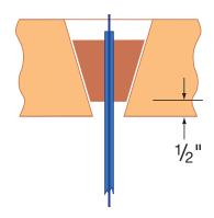
This diagram shows specimen fully engaged in grip faces and grip faces correctly supported inside grip pockets. Correct arrangement. *Photo: ADMET Inc.*
