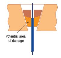
The diagram shows a specimen partially engaged in grip faces and grip faces correctly supported inside grip pockets. Arrangement can cause permanent damage to grip inserts and may lead to specimen slippage. *Photo: ADMET Inc.*
