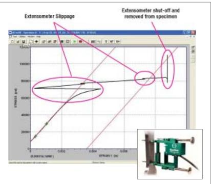
A stress-strain curve shows extensometer slippage. Inset: An extensometer is attached to a flat specimen. *Photo: ADMET Inc.*
