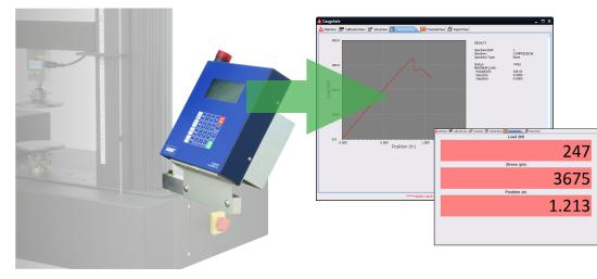
Combining the eP2 indicator with the PC based GaugeSafe software makes it easy to create and store unlimited number of test methods; save, export and print test results including stress vs. strain curves; import results and XY data into common spreadsheet and database programs for further analysis and reporting.
